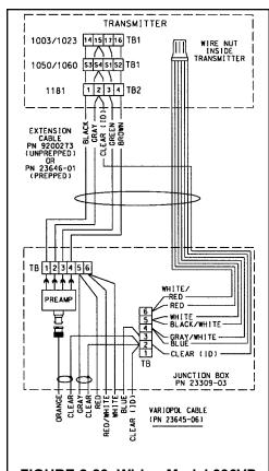
FIGURE 2-23. Wiring Model 396VP and 398VP to Model 1181, 1050/1060, and 1003/1023 through a Remote Junction Box
